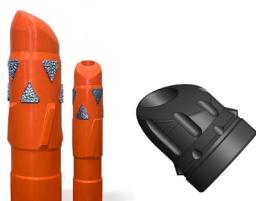
Our Razer Reamer Shoes help you get to total depth faster, no matter the obstacles. A unique eccentric nose maximizes maneuverability around obstructions and minimizes the amount of material removed during drill out. A unique design featuring Tungsten Carbide profile pads allows the reamer to pass through tight spots, while providing positive flow distribution for the debris to flow up hole and eliminate disturbances.
