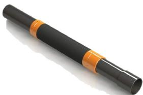
Summit inflatable casing annulus packers are suitable for cased and open hole in horizontal and vertical applications, providing a reliable, field-proven system that provides consistent zonal isolation, protection, and security. Built on a mandrel equivalent to well casing, the packer maintains burst, collapse and tensile integrity throughout the casing section, expanding to 2.5 times run-in diameter.
